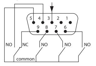
Figure 2-9: Relay Pin Connections for Communication Port.
